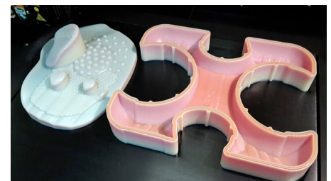
This 3D printed prototype for a swimming float was produced in full color in a mix of rigid and flexible materials, all in a single print, using the Stratasys J750 3D Printer.
