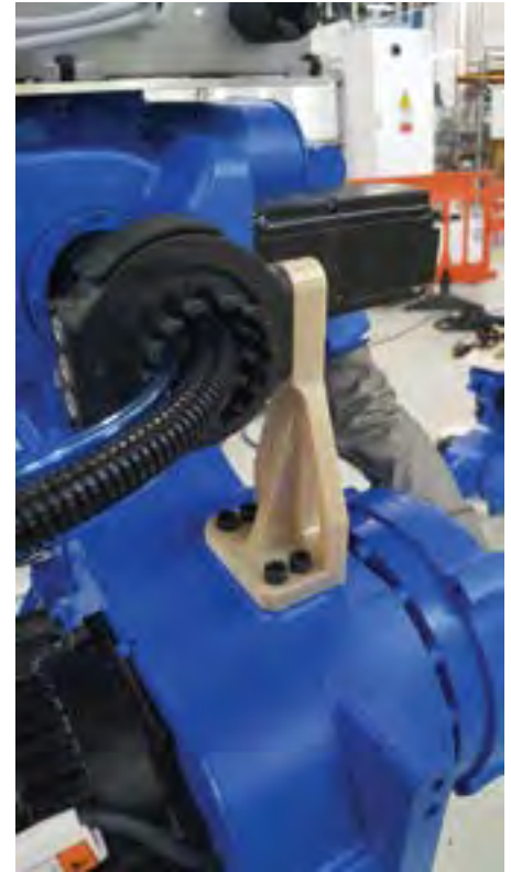
GKN Driveline Florence 3D prints replacement production parts on-demand that can endure prolonged use without fatigue.
