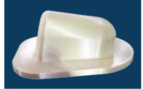
This FDM layup tool produced the aircraft camera fairings above.
