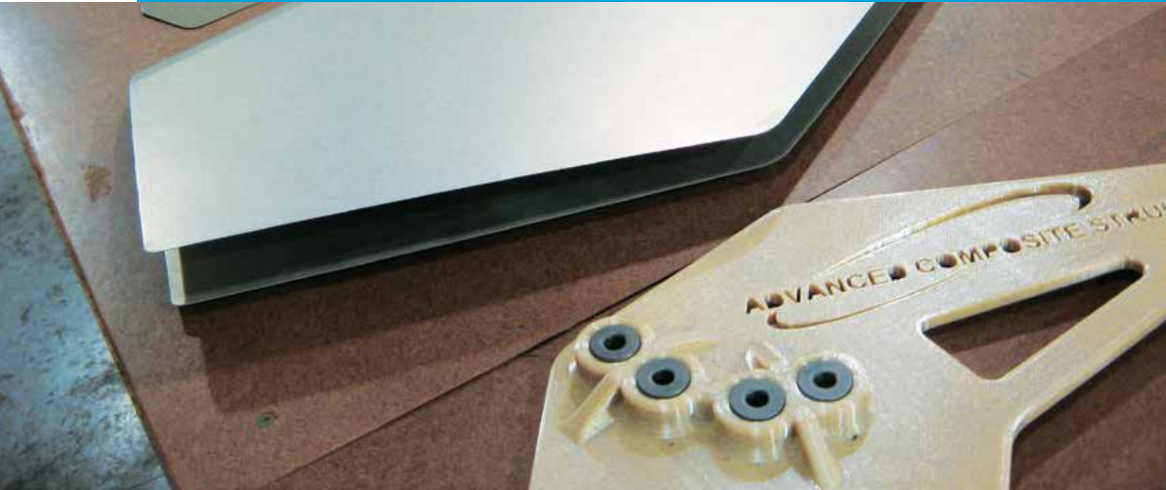
ACS used this FDM fixture as a guide to drill holes in a helicopter fin.
