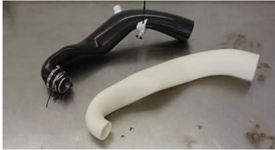
Composite turbo inlet duct (black) made using FDM soluble core (white).
