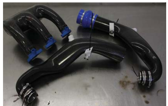
An array of complex, composite ducts made using FDM soluble cores.
