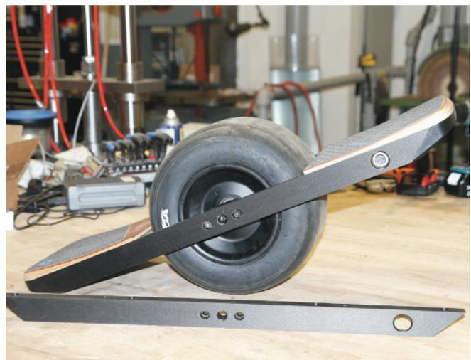
A Onewheel board with carbon fiber nylon (FDM Nylon 12CF) side rails.
