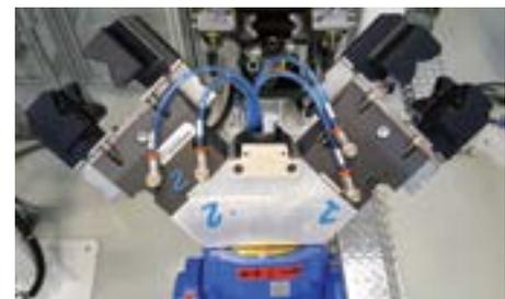
GKN Driveline Florence is testing a range of new tooling applications on their Fortus 450mc, including bespoke end-of-arm tools.
