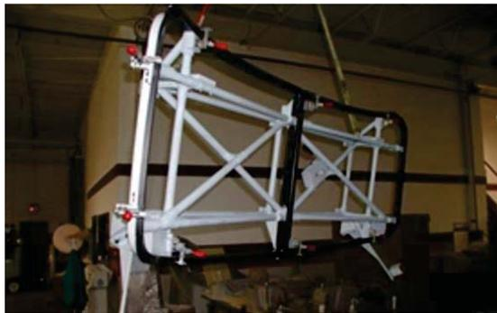
A cut-and-weld fixture for carrying a formed part.
