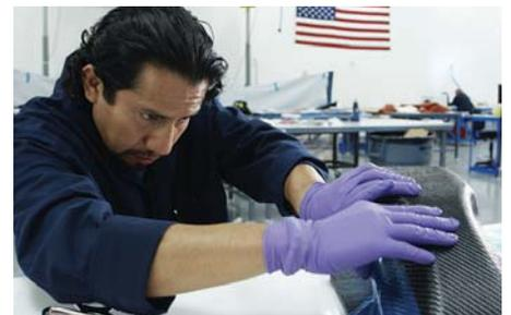
Prior to bagging for cure, the ply lay-up is completed.
