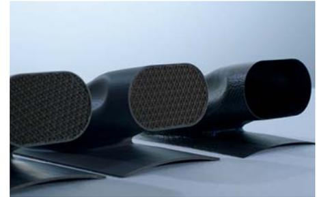
(Left to right): 3D printed tool as-built, sealed tool and final resulting part.
