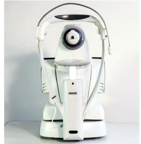
The assembled Gonioscope® prototype, built with 3D printed parts.
