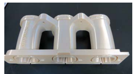
This 3D printed air aspiration engine conduit was produced in ULTEM 9085 resin on a Fortus 400mc 3D Production System.
