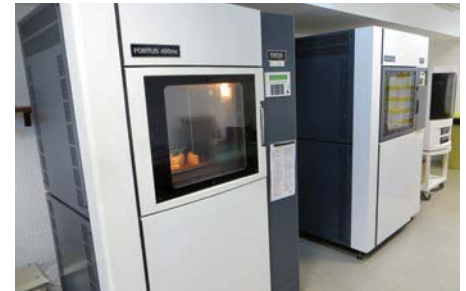
The Fortus 400mc 3D Production System produces parts that include Nolders, an aerodynamic profile installed under vehicle bumper.
