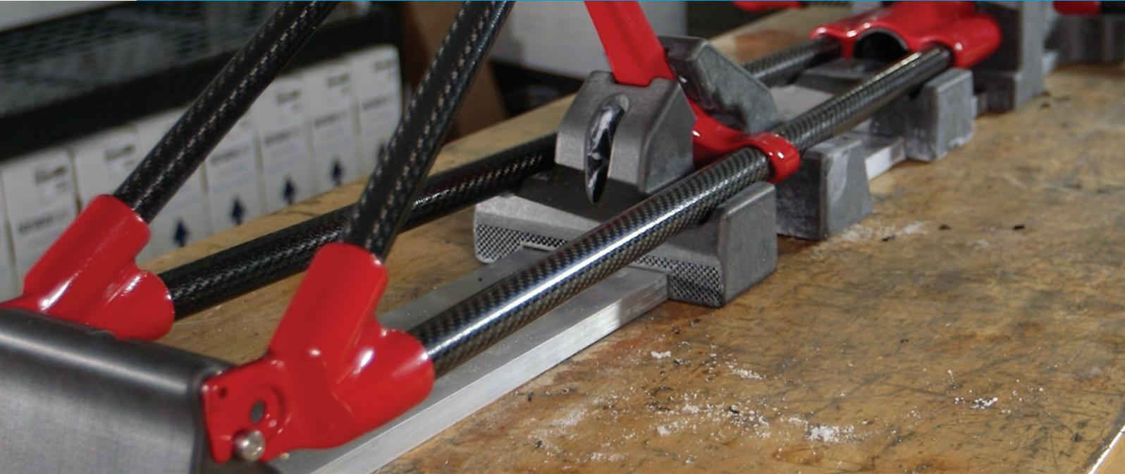
These custom lugs, made with Stratasys FDM Nylon 12CF, are painted red after emerging from the tumbler with a smooth, polished finish.
